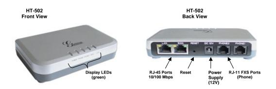
The HT502 has 2 FXS port. Both FXS ports can have a separate SIP account. This is a key feature of HT502 as it supports <u>simultaneous</u> calls on both FXS ports.
