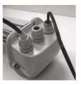
12. Remove the terminal block. Plug black and white wires of the power cable to the terminal block. Reinsert the terminal block onto the camera. The white wire is required to connect to the positive pin (+) on the camera and the black wire to the negative pin (-).
