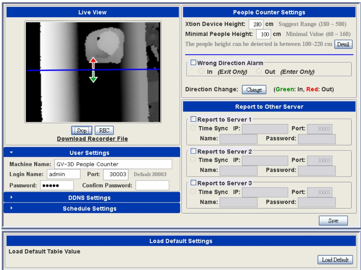
The screenshot shows the 'Detection Setting' page for a GV-3D People Counter. It features a 'Live View' window on the left showing a grayscale camera feed with a blue detection line and red/green arrows indicating direction. Below the live view are 'Stop' and 'REC' buttons, and a 'Download Recorder File' link. The main settings area is titled 'People Counter Settings' and includes:
