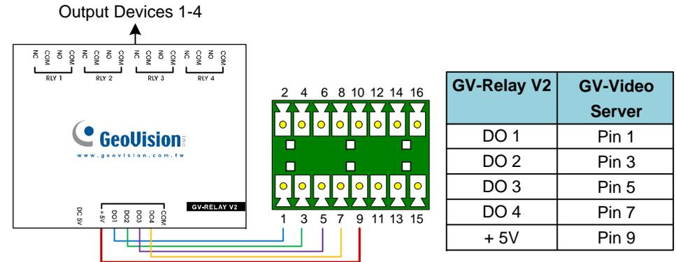
**Note:** You don't need to use the DC 5V connector on the GV-Relay V2 for power supply, since the power is supplied from the GV-Video Server or GV-DSP LPR.
