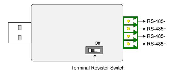
**Note:** The GV-COM V2 is only capable of converting one RS-485 signal. The RS-485 port on the GV-COM V2 is extended into two sets of connection points.
