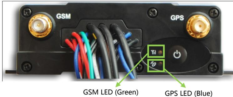
Press and hold the Power On/Off button for 3~5 seconds to turn on/off MVT800.
