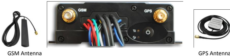
Connect the GSM antenna to the SMA connector which is 'GSM' text labeled. The GSM antenna is non-directional, so you can hide it in any place of vehicle.
